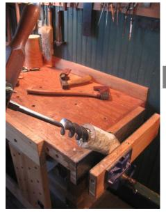
First, bore a hole through the center of a fresh green branch section.
